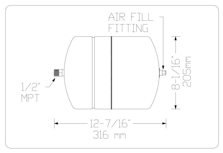
MAXIMUM WORKING PRESSURE: 100 PSIG FACTORY PRE-CHARGE PRESSURE SETTING: 12 PSIG MAXIMUM WORKING TEMPERATURE: 212° F / 100° C WEIGHT: 5.0 LBS / 2.3 KG
